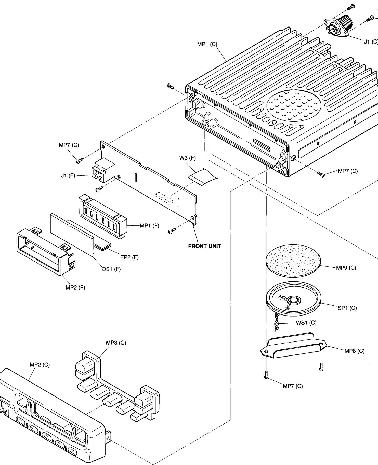
**Unit abbreviations** (F): FRONT UNIT (M): MAIN UNIT (C): CHASSIS PARTS
