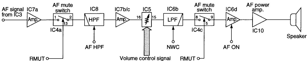
A portion of the AF signals from the AF amplifier (IC7a) passes through the low-pass filter (FRONT unit; Q5) to remove AF (voice) signals and is applied to the CTCSS or DTCS decoder inside the CPU (FRONT unit; IC1, pin 97) via the "CTCIN" line to control the AF mute switch via the I/O expander IC (IC11).
