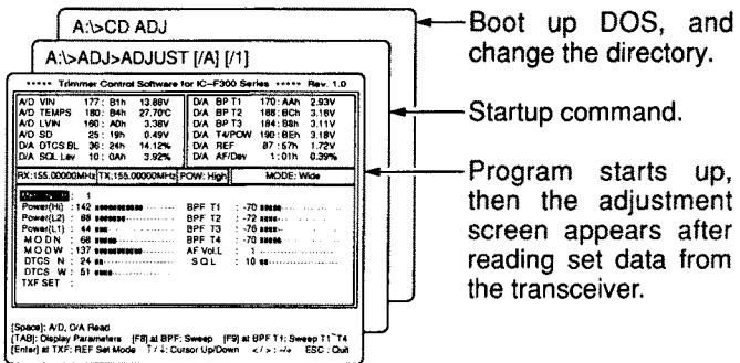
**NOTE:** When the EEPROM (FRONT unit; IC3) is replaced or the transceiver displays an error message and beeps, the following operation is necessary before starting the ADJUSTMENT.
